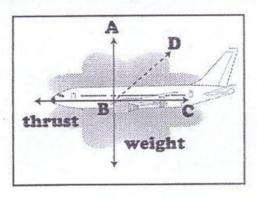
In the figure above, the difference between the above-wing pressure and the below-wing pressure results in the force BD.
