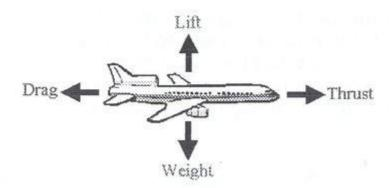
A force may be thought of as a push or pull in a specific direction. A force is a vector quantity so a force has both a magnitude and a direction. When describing forces, we have to specify both the magnitude and the direction. This picture shows the forces that act on an airplane in flight.
