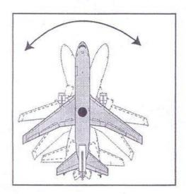
An aircraft is trimmed to ensure stability. During take-off and landing, trimming is a constant process, while in cruise it is usually performed automatically by computers. The horizontal stabilizer may be computer-controlled, with the appropriate setting determined by the computer in light of flight parameters.
